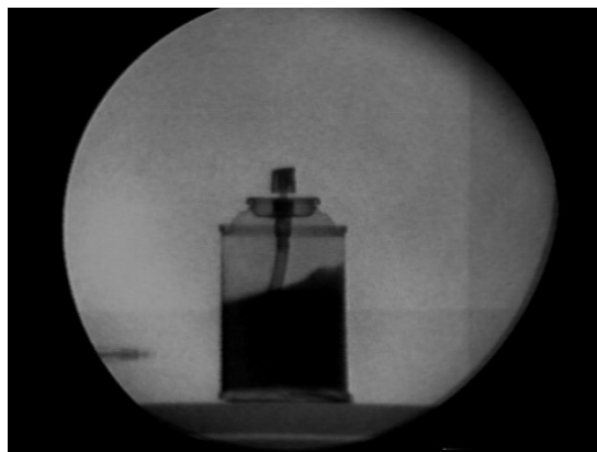
Figure 2: Neutron Radiograph of a Spray Paint Can Captured in Motion
